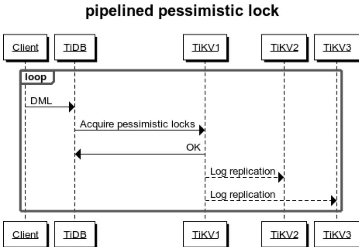
图 492: Pipelined pessimistic lock
