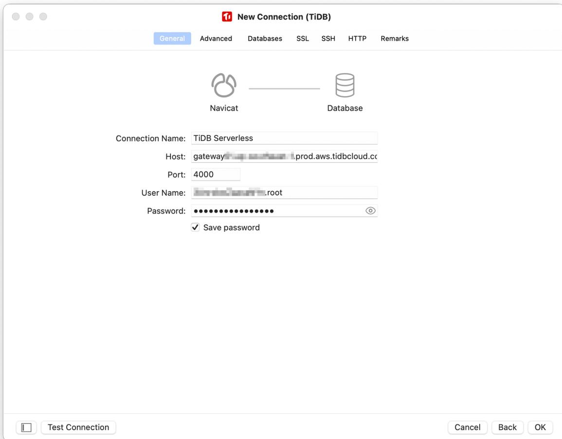
图 12: Navicat: configure connection general panel for TiDB Serverless
