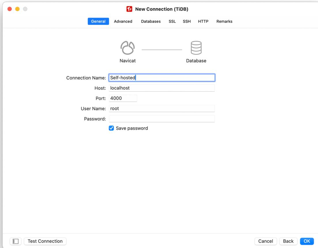
图 18: Navicat: configure connection general panel for self-hosted TiDB
