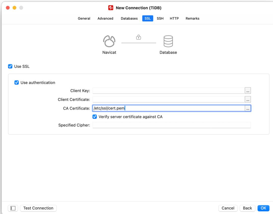
图 13: Navicat: configure connection SSL panel for TiDB Serverless
